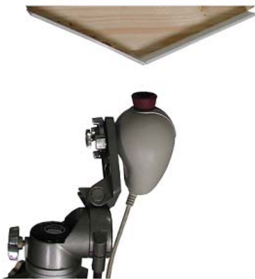
Figure 4: Two-way vision by placing two mirrors above a vertically aligned webcam.
