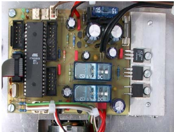
Fig.10: Power board with Atmel controller
