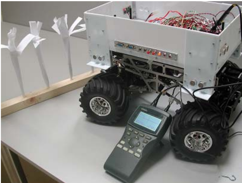
Figure 7: Measuring sonar response with an Oscilloscope
