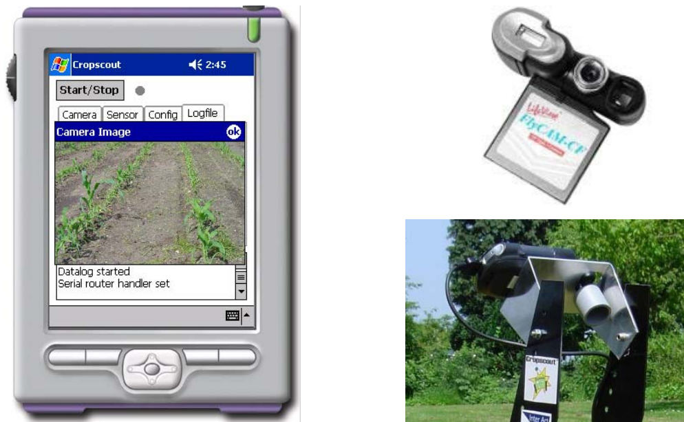
Figure 6. Graphical user interface of pocket PC used for camera vision based row detection and navigation (left), the FlyCAM CF camera (top right) and close-up of the camera construction with wide-angle lens (bottom right).
