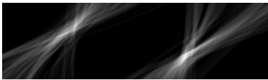
Figure 3. Hough-space. Horizontal coordinate denotes the point at which a line crosses the top of the image in Fig. 2; vertical coordinate denotes the angle of the line; brightness denotes the number of white (crop) pixels on the line.
